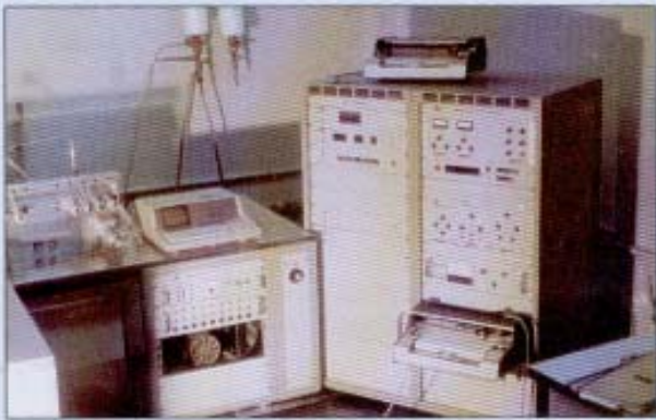
Mass spectrometer for measurement of stable isotopes of water
