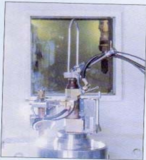
Remote Welding of Vitrified Waste Canister at Waste Immobilisation Plant, Trombay
